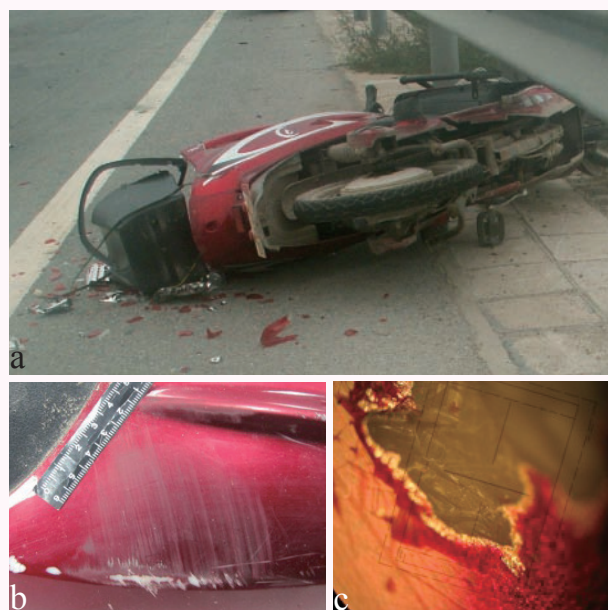
Figure 1: (a) Photograph of the red motorcycle; (b) damage mark on the back cover; (c) the paint layers on a white polymeric substrate of the red motorcycle under magnification.
