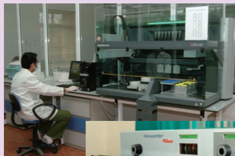
Robot system (TECAN) for DNA Liquid handling in the national DNA database of criminals.
